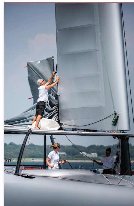
The hybrid mainsail consists of a fixed wing attached to the mast and a sailcloth section for the relevant weather. An attractive but demanding process in terms of sail handling.
