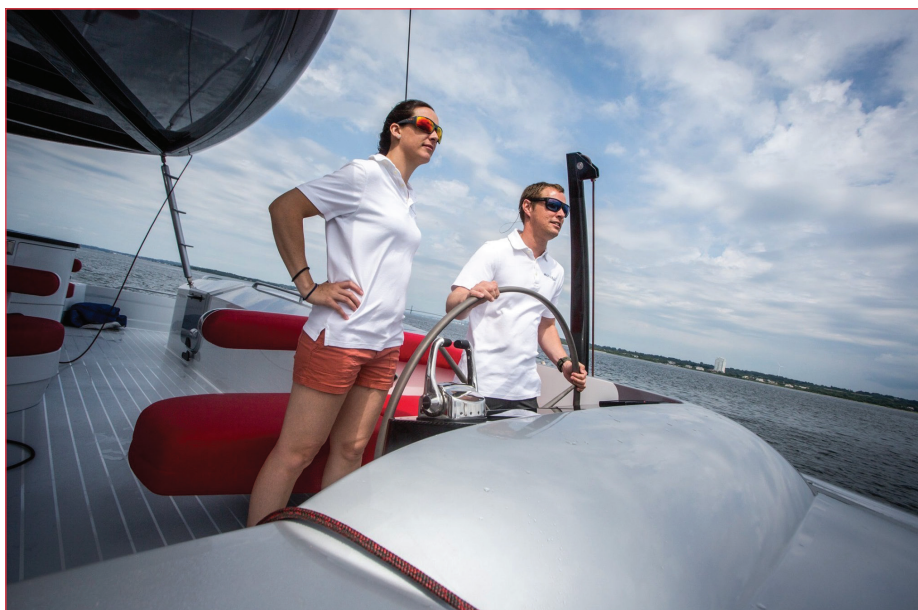
The twin helm stations, which are set well forward, free up the cockpit and offer a totally unobstructed view of the water and the sails.
